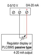
Connection of output in voltage 0-10 V:
